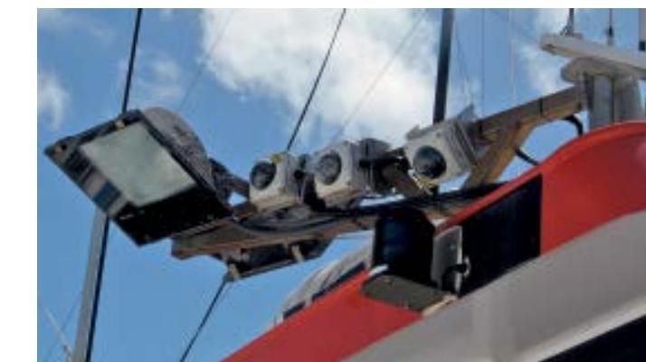
on and record the longline gear being both set and hauled in. The GPS receiver is in addition to AFMA's existing Vessel Monitoring System (VMS), a satellite-based automatic location communicator, which is a mandatory requirement for all Commonwealth commercial fishing vessels.
